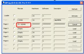
Uploading into the first page is in progress. 10 fragments of 448 are uploaded.
