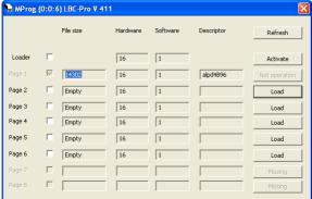
The above example demonstrates the status of memory pages in the LCB located in Slot 6 of Nodal Unit 0, Subnet 0. An active firmware is loaded into the first page, i.e. it is currently running.
